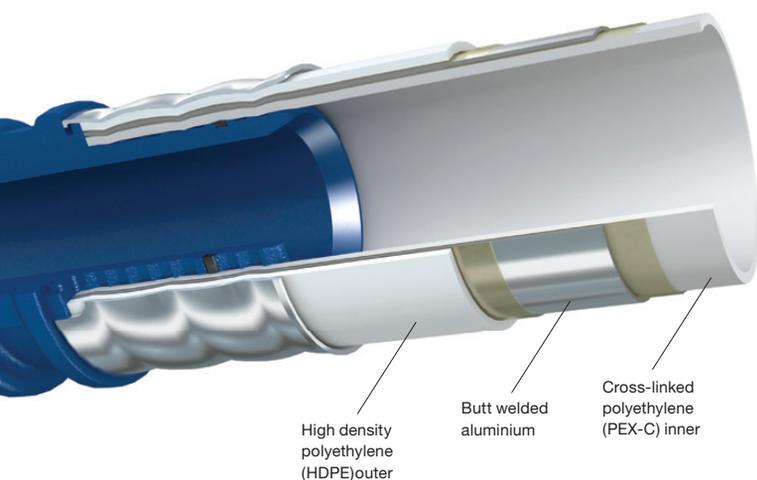
The multi-layer pipe is integral to the exceptional performance of Tigris K1, uniting the benefits of metal and plastic into one composite solution. The pipe comprises an inner plastic layer of cross-linked polyethylene, an outer plastic layer of HDPE and a butt welded aluminium layer in between.
